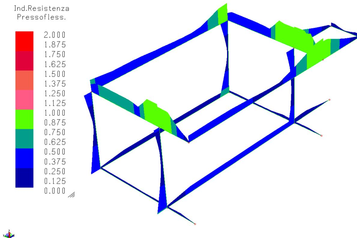
Indice di resistenza a taglio e torsione
