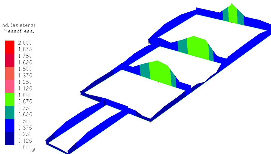
Indice di resistenza a taglio e torsione
